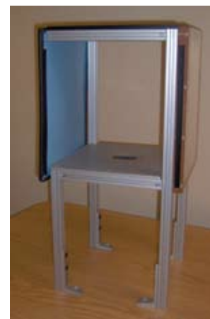
The benchtop test stand's leaded glass shielding provides full view of the test chamber while guarding against radiation exposure.
