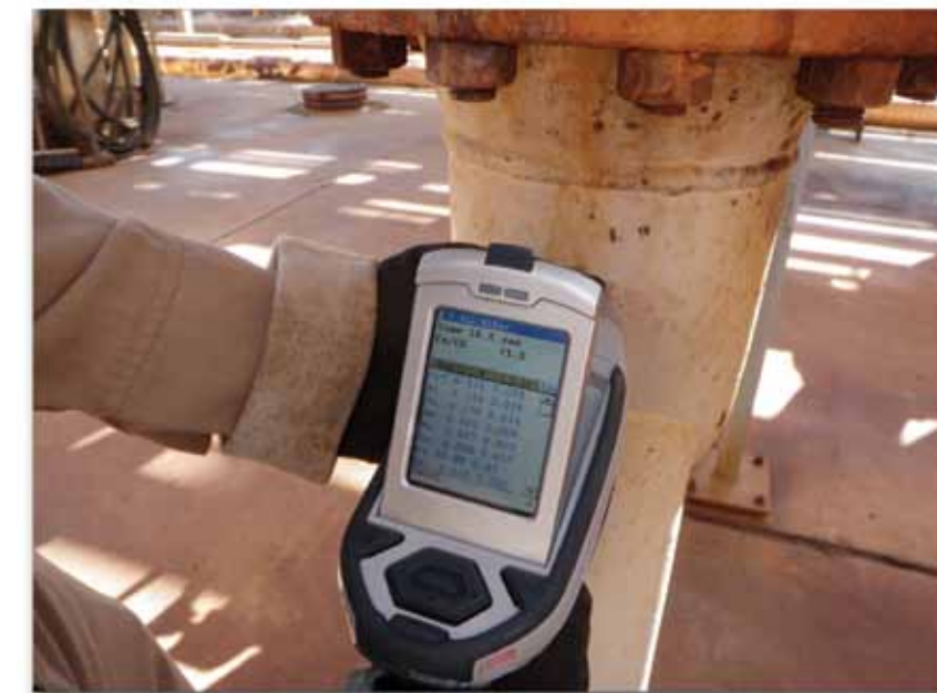
The elemental composition of a CS pipe in an HF alkylation unit at a Texas refinery is displayed on the screen of a handheld XRF analyzer. Photo courtesy of Thermo Fisher Scientific.
