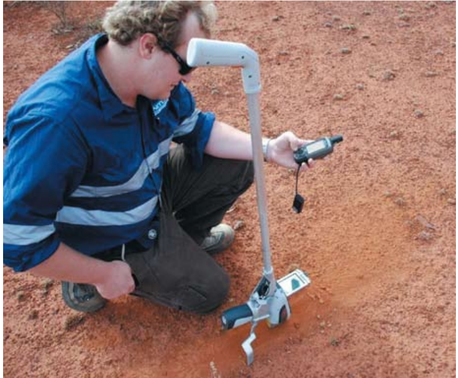
In-Situ NITON XRF unit soil testing with a global positioning unit.
