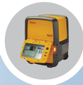
Small-spot feature: Isolate test areas as small as 1 mm and conveniently store sample measurements for later reference.
