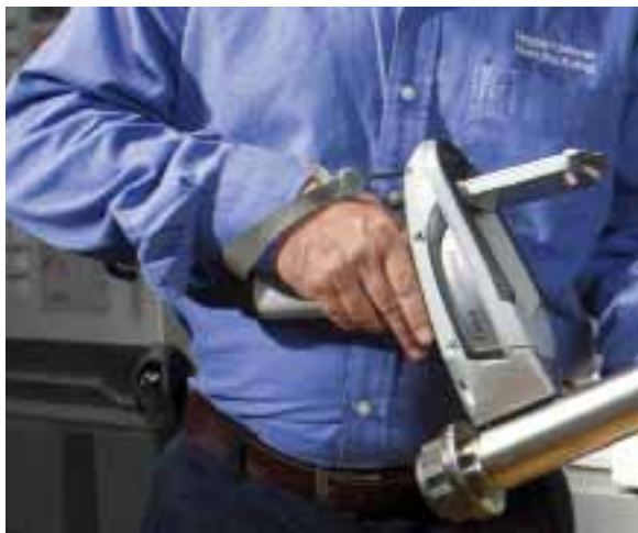
Material verification using the Niton XL3t analyzer
