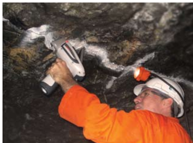
The Thermo Scientific Niton XL3t 500 is an ideal instrument for fast mine or field analysis.
